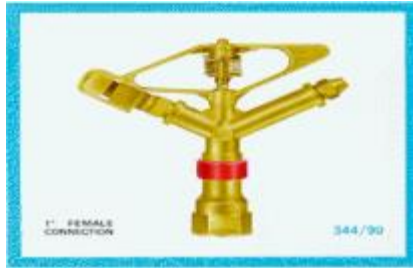
NAAN 344/90 MAJOR SIZE General Purpose Sprinkler. With two nozzles, larger discharges and precipitations. Spoon hammer drive, thrust spring and protector sleeve, stainless steel axle. Weight: 770 g
