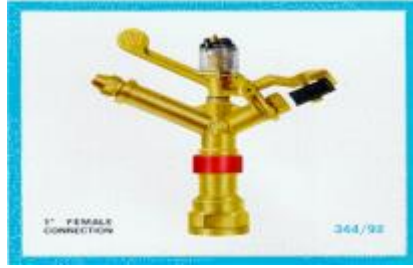
NAAN 344/92 MAJOR SIZE General Purpose Sprinkler. Brass hammer, wedge drive, thrust spring and protector sleeve, stainless steel axle. Weight: 730 g
