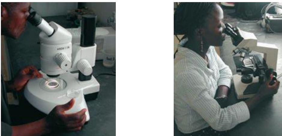
Figure 7: Viewing nematodes under dissecting stereomicroscope (left) and compound microscope (right)
