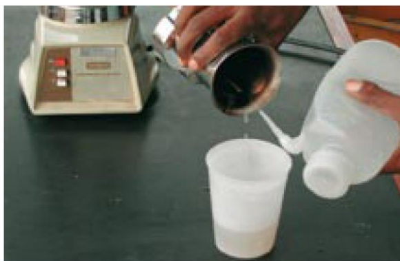
5. Pour blended suspension into a labeled beaker and rinse out blender into the beaker.
