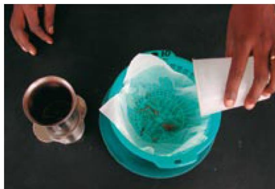
6. Gently pour the sample onto the tissue paper in the sieve as for extraction tray method.
