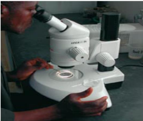
Using a dissection stereo-microscope with understage lighting.
