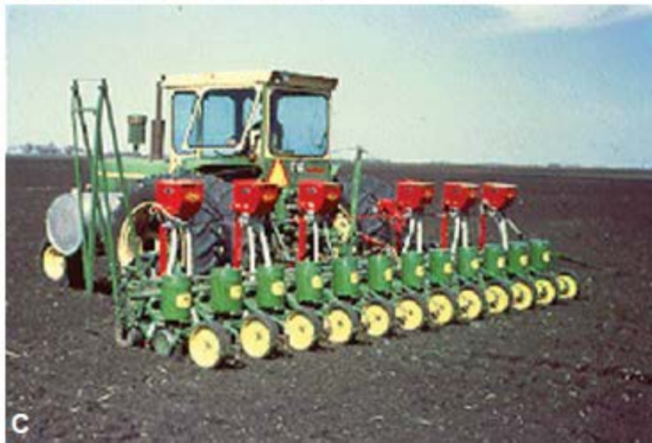
FIGURE 9-31 Equipment for application of soil pesticides and fumigants. (A) Tractor applying a fumigant and laying plastic over it to keep the chemical from early escape. (B) Field beds treated with a volatile chemical and covered with plastic. (C) Multidisk tractor used to incorporate nonvolatile granular chemicals in soil. (D) Broadcast chisel application of low-volatility liquid fumigants into soil. [Photographs courtesy of (A) R. T. McMillan and (B–D) D. W. Dickson, University of Florida.]
