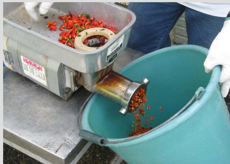
Pepper seed extraction using a grinder
