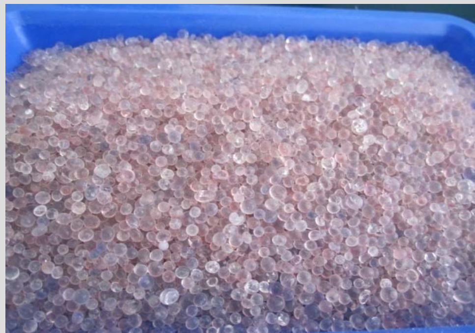
Silica gel turns pink after water adsorption from seed
